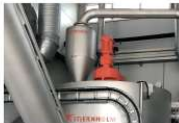
Capacity of the sand washer can be increased by mounting a cyclone at the inlet.
