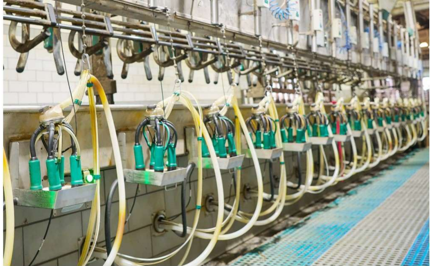
DairyProX is a semi-automated milking system designed to fit into your current conventional parlor. Everything looks and feels the same at the operator level, and the technology resides out of the way in the subway.
